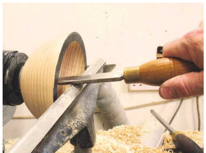
▲ Pic.7 The scraper is a good tool if you're struggling to get the centre of the bowl right. I have put the toolrest close to the bowl to give the cutting edge as much support as I can
